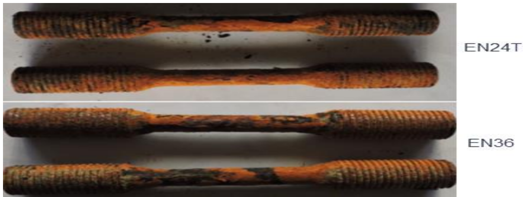
Figure 3. Test specimens after 1000 hours of exposure
