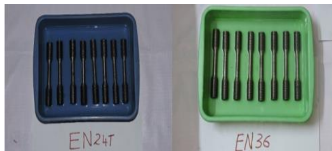
Figure 2. Test specimens immersed in sea water
