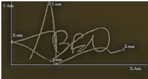
Figure 5. Computation of Xmin, Xmax, Ymin and Ymax.
