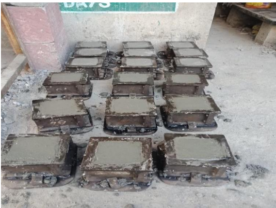
Fig. 1 Concrete Cube Moulds
