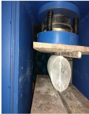
Fig. 6 Split Tensile Testing
