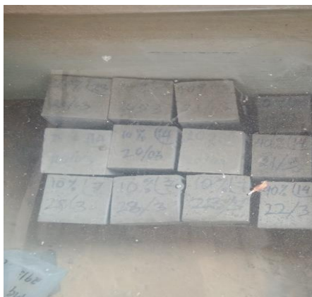
Fig. 3 Curing of Concrete Cubes
