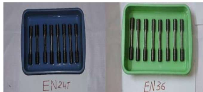
Figure 2. Test specimens immersed in sea water
