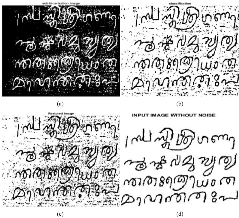
Figure 5 (a) Sub-binarised image (b) Newly binarised image B3 (c) Restored image (d) Enhanced binary image
