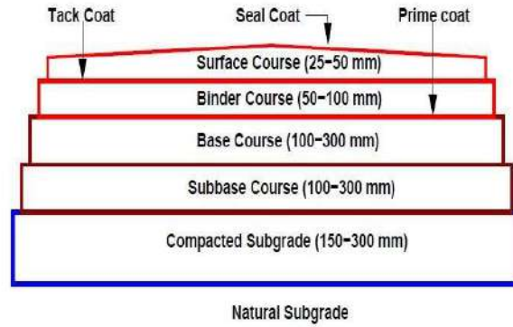
Typical cross section of a flexible pavement
